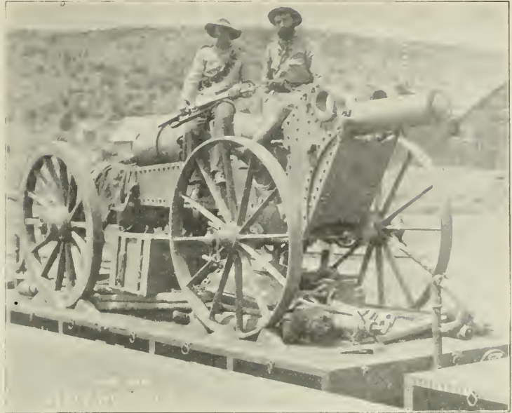
THE RESTORED GUN LONG TOM. During the night of 8 December 1899, one of the guns, Long Tom, which bombarded Ladysmith, was rendered useless by the British. A charge of dynamite placed in the muzzle did great damage. But the destruction of the gun was by no means complete, and it was easily repaired. Long Tom was ready for work again in a very short time, and was dispatched by rail to Ottoskop, near Kimberley. The gun created no little dismay among the inhabitants of the latter city.
